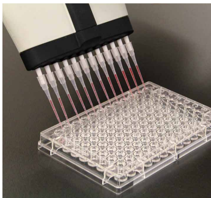
Figure 2. Micro-pipetting with 10µl Long Reach Tips for precision pipetting
