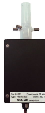
NO 2 and NO 3 Reactor
