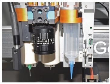
Head tools on Z-drives. From left to right: heated cartridge + UV optical fibre, heated cartridge + camera, normal cartridge (30 ml), piezo pipette.
