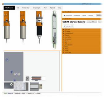
Control app with print head and workspace configuration (left), and tabs for tool definition (right). The Generator button is to create simple geometric forms.
