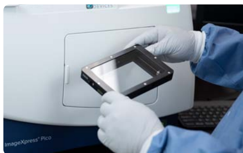
Magnetically sealed environmental control cassette reduces gas usage
