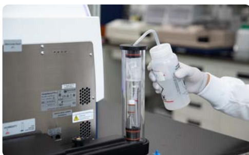
Integrated humidity column is easily refilled without disrupting ongoing experiments
