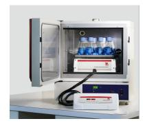
The extended ribbon cable (1.68m) can easily pass underneath an incubator door or via incubator's utility port, for external control. Avoid unnecessary disruption of the internal environment.
