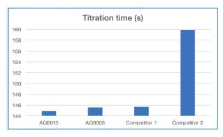
Another important point when choosing a one-component Karl Fischer reagent is the titration speed. In the following table, we can see that the titration velocity of the new Aquagent® Complet 5 is one of the fastest on the market, improving on that of Scharlau's previous formulation.
