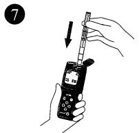
Insert the whole body of the Luci-Pac into the measurement chamber of Lumitester. And close the chamber cover.
