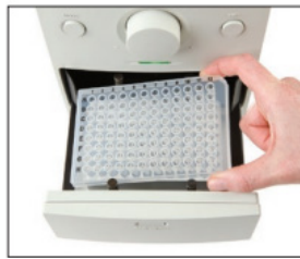
1. Open drawer and insert plate.
